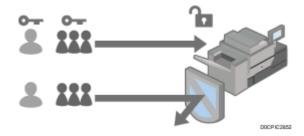
User authentication prevents unauthorized users from operating the machine and is useful for managing and analyzing usage of the machine regarding the user, operation time, and frequency.
